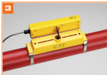
Connect power and sensors to electronic assembly
